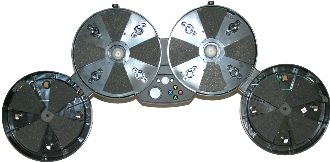
All the drum pads removed
